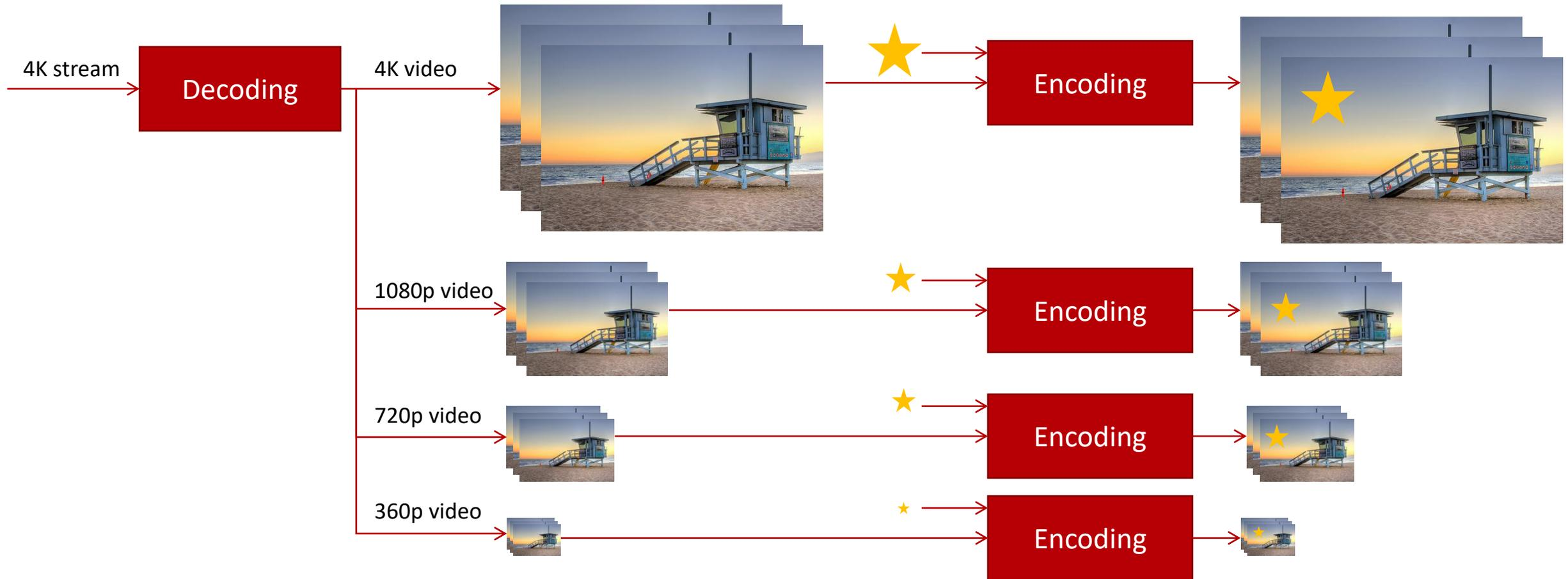
Decoder can support up to 4 resized outputs (down scaling and up scaling)
