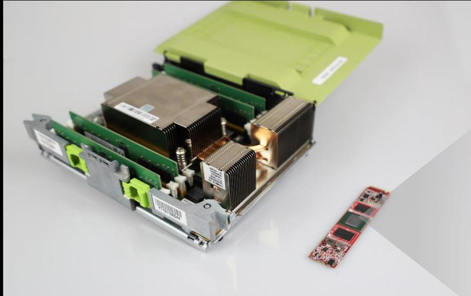
CPU vs Video transcoding ASIC
